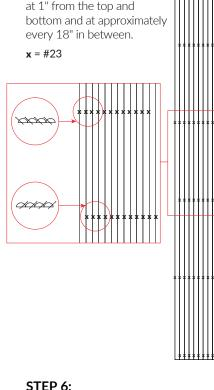
Installation of subsequent panels: Repeat step 1, 2 and 3, align against the installed wall panel and gently roll into place, repeat step 5 and so forth.
