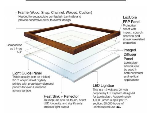
Lumisplash is available in kit form with all necessary hardware supplied for installation. This all-in-one contained system saves time and money compared to other products that require extensive fabrication and set-up or bulky bulbs and wiring.
